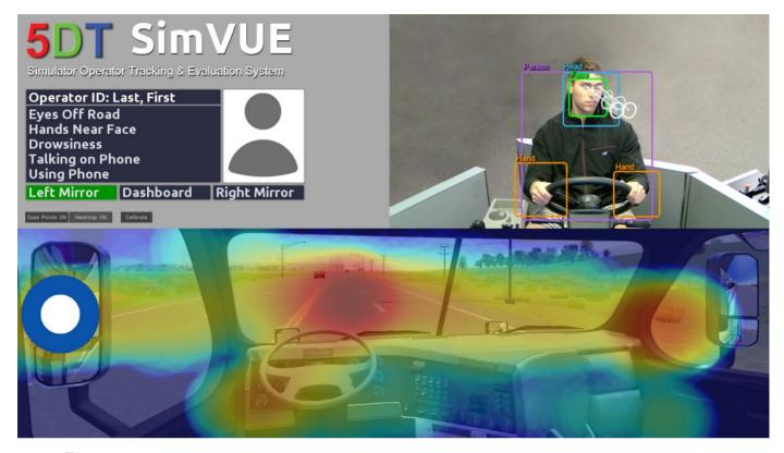
SimVUE™ with heatmap functionality turned on. The heatmap shows the dwell time of the simulator occupant's gaze point. The simulator occupant is checking his left mirror. Both the operator's hands are on the steering wheel.
